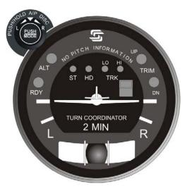
Fig. 2-2. AP Display, All Lamps Extinguished (System Twenty)
