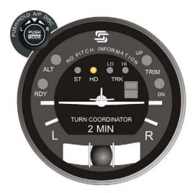
Fig. 3-2. AP Display, HD Mode Engaged
