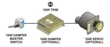
Fig. 1-4. Yaw Damper Block Diagram
