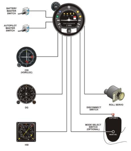
Fig. 1-1. System Twenty Block Diagram
