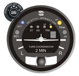
Fig. 2-26. AP Display, HI TRK and ALT HOLD Modes Engaged, TRIM UP Required (System Thirty)
