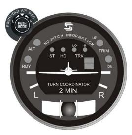
Fig. 2-9. AP Display, All Lamps Extinguished (System Thirty)
