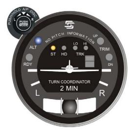
Fig. 3-5. AP Display, ST and ALT HOLD Modes Engaged (System Thirty)
