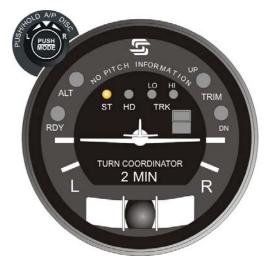
Fig. 2-21. AP Display, ST Mode Engaged (System Thirty)
