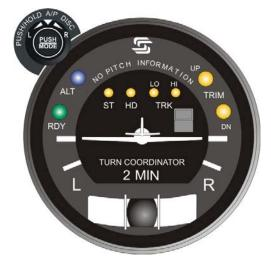
Fig. 2-6. AP Display, RDY, ALT, ST, HD, LO TRK, HI TRK, TRIM UP, TRIM DN Lamps Illuminated at Power-Up (System Thirty)
