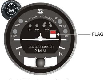
Fig. 2-5. AP Display, Low Voltage Flag (System Twenty)
