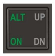
Fig. 2-15. ALT HOLD ON/OFF Switch Display, DN Lamp Extinguished (System Thirty ALT)
