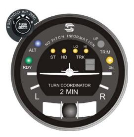
Fig. 2-7. AP Display, TRIM UP Lamp Extinguished (System Thirty)
