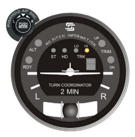
Fig. 2-24. AP Display, HI TRK Mode Engaged (System Thirty)
