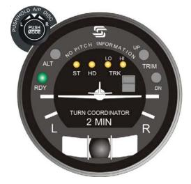
Fig. 2-1. AP Display, RDY, ST, HD, LO TRK, HI TRK Lamps Illuminated at Power-Up (System Twenty)
