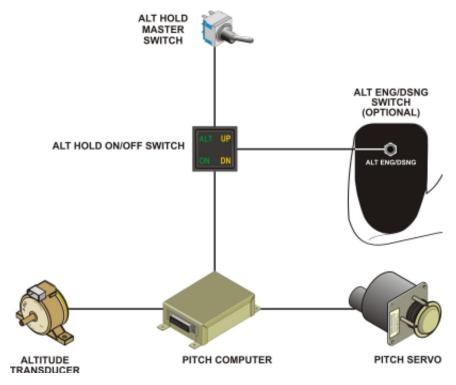
Fig. 1-3. System Thirty ALT Block Diagram
