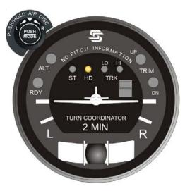
Fig. 2-22. AP Display, HD Mode Engaged (System Thirty)
