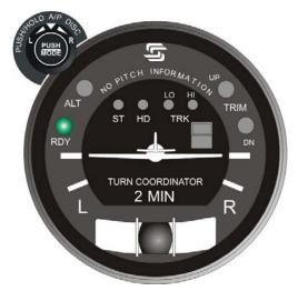
Fig. 2-3. AP Display, RDY for Operation (System Twenty)
