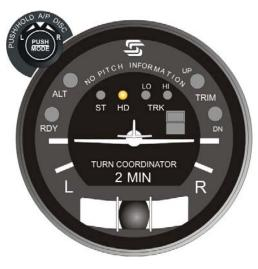
Fig. 2-18. AP Display, HD Mode Engaged (System Twenty)
