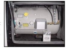
Figure 2-4. Liquid Propane Tank
