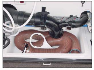
Figure 11-14. Sewer Hose and Drain Connections
