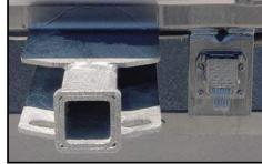
Figure 2-8. Class 3 Towing Hitch
