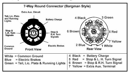
Figure 7-20. Bargman 7-Way Round Towing Connector
