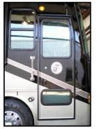
The primary entrance door (Figure 13-5) to the motor home is a radius door having a key lock and a dead bolt for additional security. When the door is fully opened, the door hinge automatically holds the door in an "open" position.
