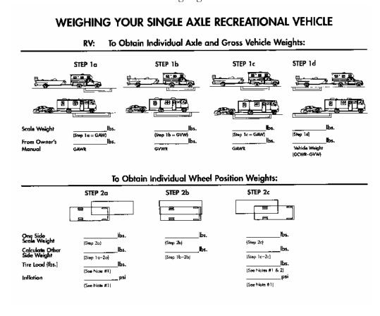
Figure 14-7. Procedure for Weighing the Motor Home (Each Tire Position Individually)
