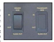
Figure 8-1. Slide-Out Switches
