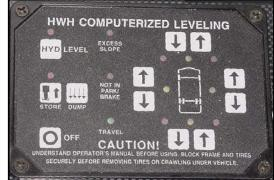
Figure 9-5. HWH Computerized Leveling System
