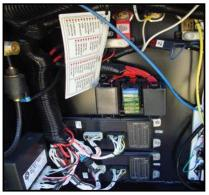
Figure 7-2. 12 VDC Fuse Panels
