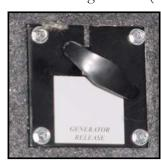
Figure 7-18. "Pull" Cable for Generator Release
