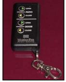
Figure 13-3. Dometic Awning Key Fob Controller
