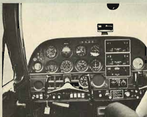
Entire instrument panel is biased toward the left, with all gauges centered in front of pilot. Vent window can open up to 120-mph.
