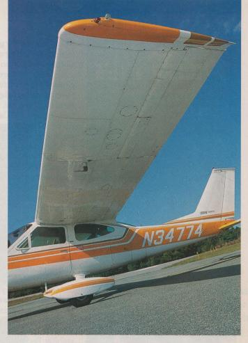
The sleek Cardinal wing and low-slung fuselage gives the Cardinal a modern look that it retains decades after its introduction. The Cardinal's panel was designed with plenty of room for avionics, though the large clunky-looking Cessna ARC radios that were standard in the airplane gobbled the space up quickly.
