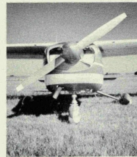
That smooth aluminum-and-fiberglass cowl has a different shape from the Skyhawk and sports only one exhaust stack — which means there's a four-cylinder Lycoming inside.
