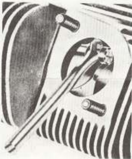
Figure 2. View Through Exhaust Port Showing Mechanical Fingers Supporting Exhaust Valve Away From Guide
