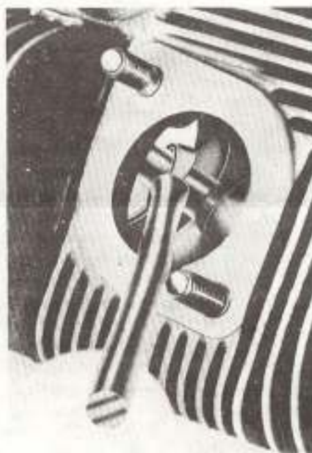
Figure 1. View Through Exhaust Port Showing Mechanical Fingers Holding Valve Stem
