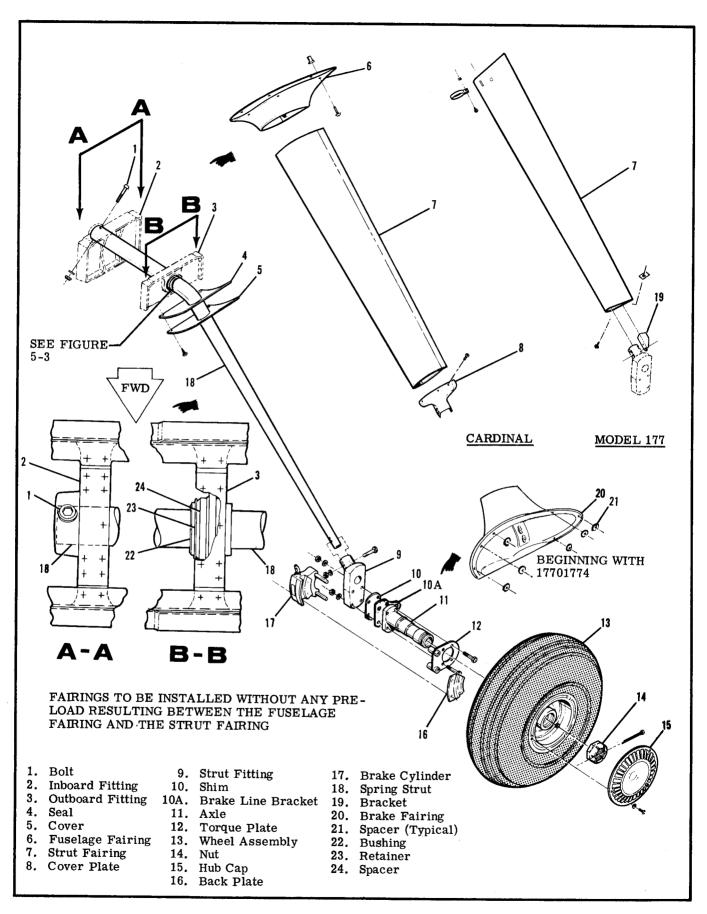
Figure 5-1. Main Gear Installation
