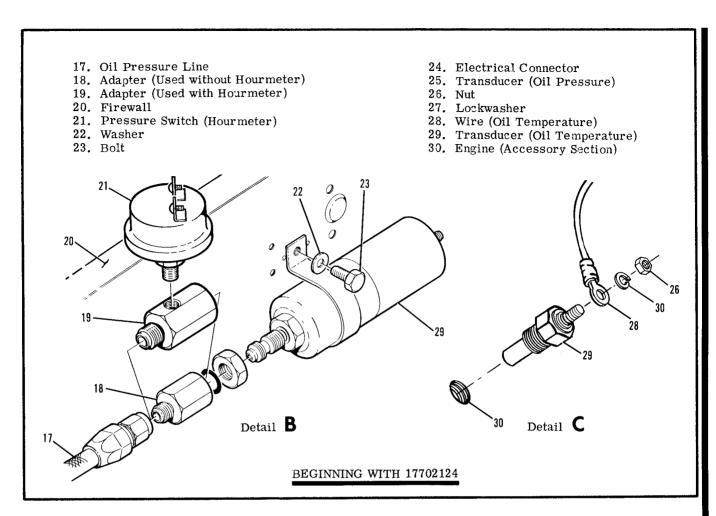
Figure 15-5A. Engine Instrument Installation (Leigh System) (Sheet 2 of 2)
