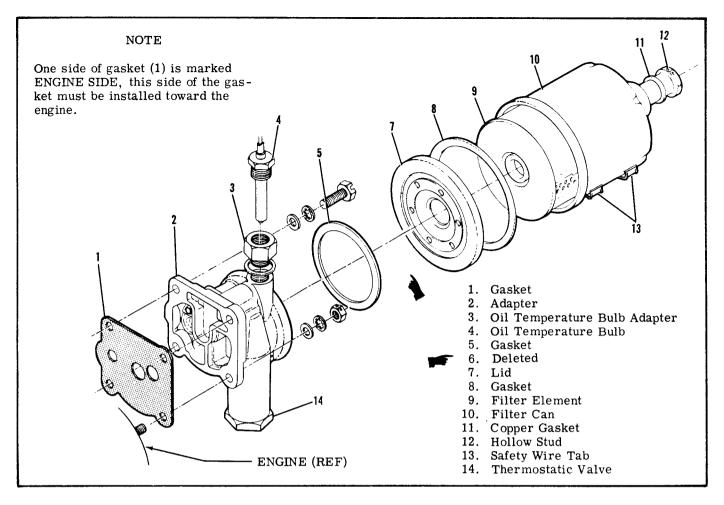
Figure 11-3. Full-Flow Oil Filter
