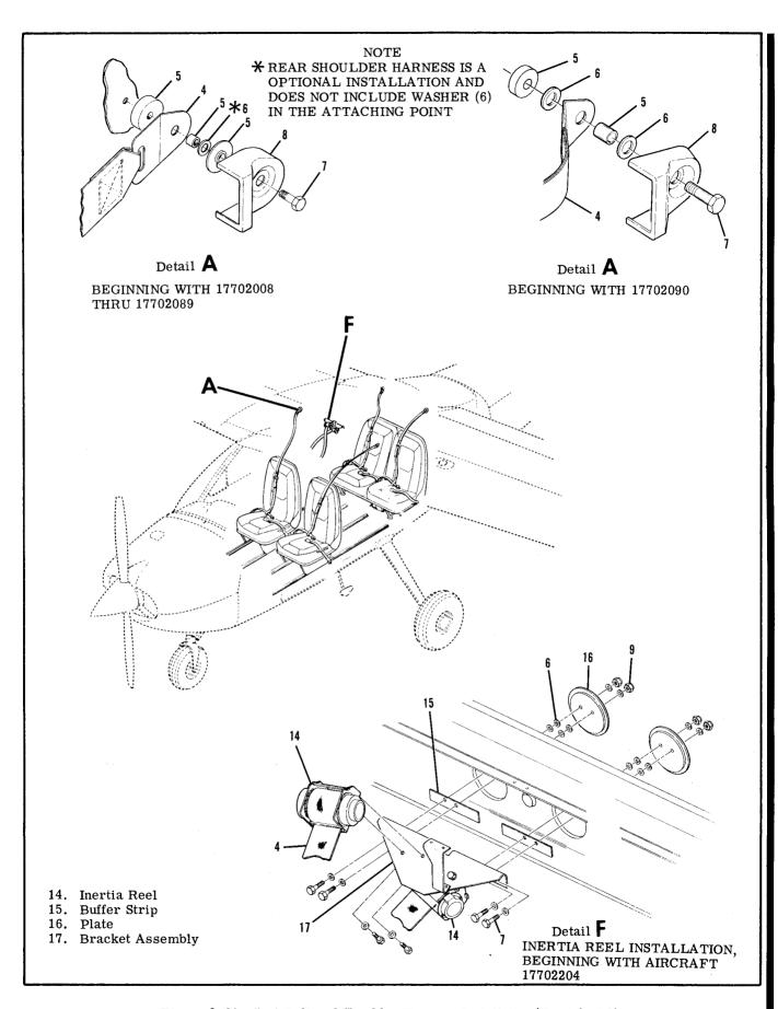
Figure 3-6A. Seat Belt and Shoulder Harness Installation(Sheet 2 of 2)
