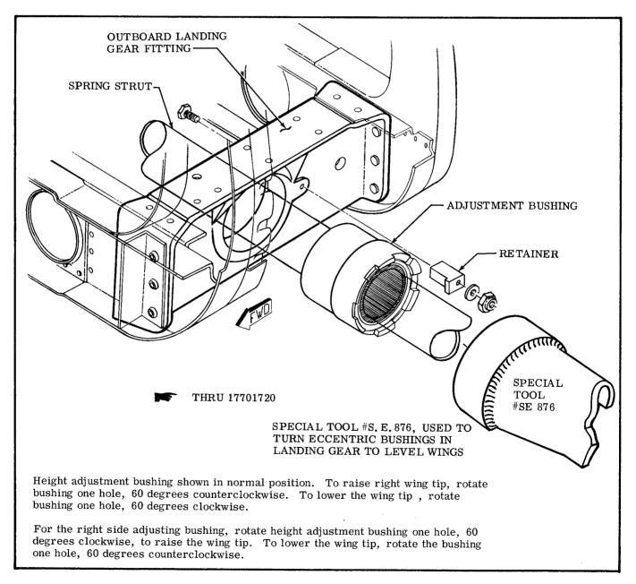
Figure 5-3. Wing Tip Height Adjustment
