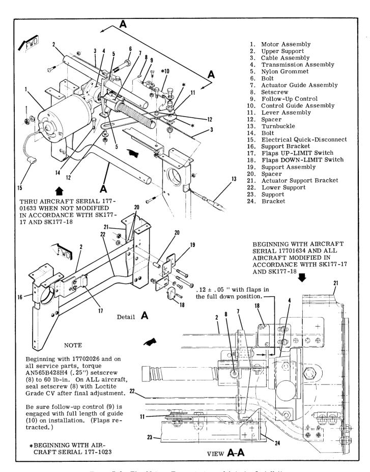
Figure 7-2. Flap Motor, Transmission and Actuator Installation
