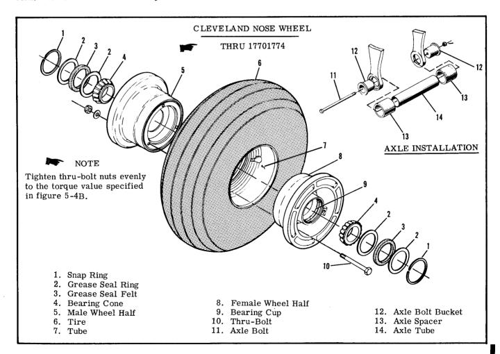
Figure 5-8. Nose Wheel (Sheet 1 of 3)
