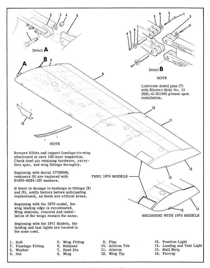
Figure 4-1. Wing Installation
