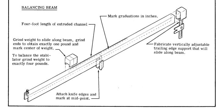
Figure 18-3. Control Surface Balancing (Sheet 1 of 4)
