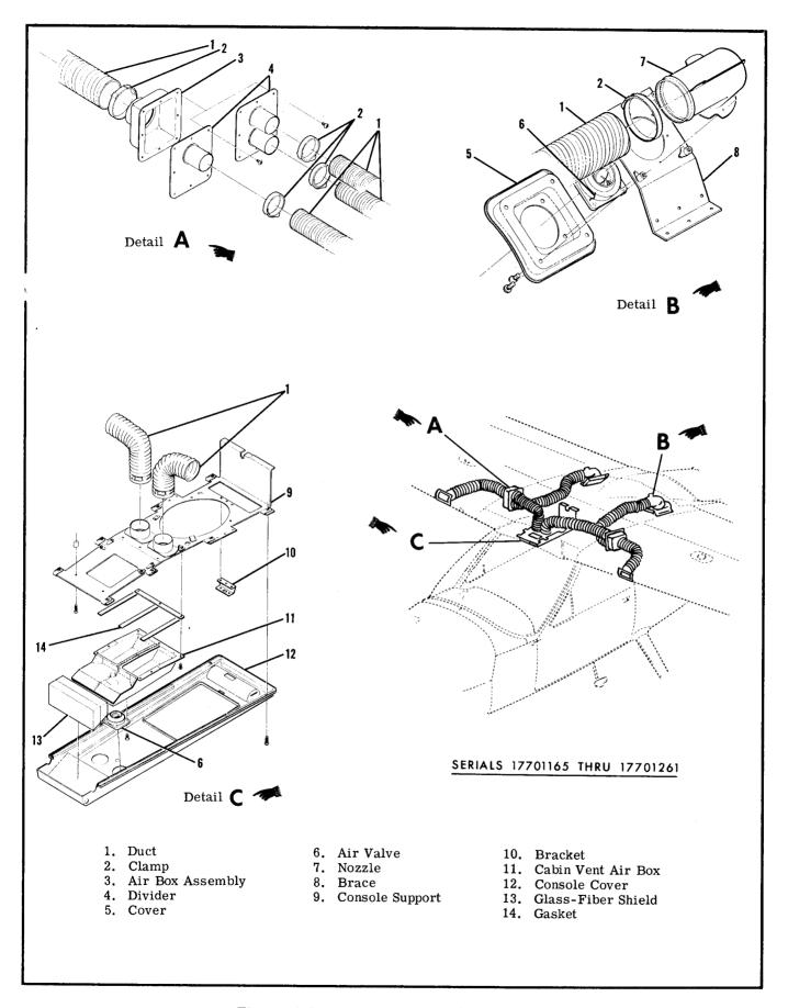
Figure 14-2. Ventilating System (Sheet 2 of 3)
