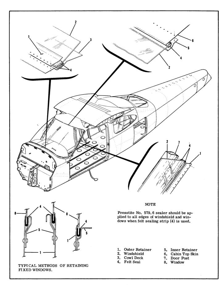
Figure 3-2. Windshield and Fixed Window Installation
