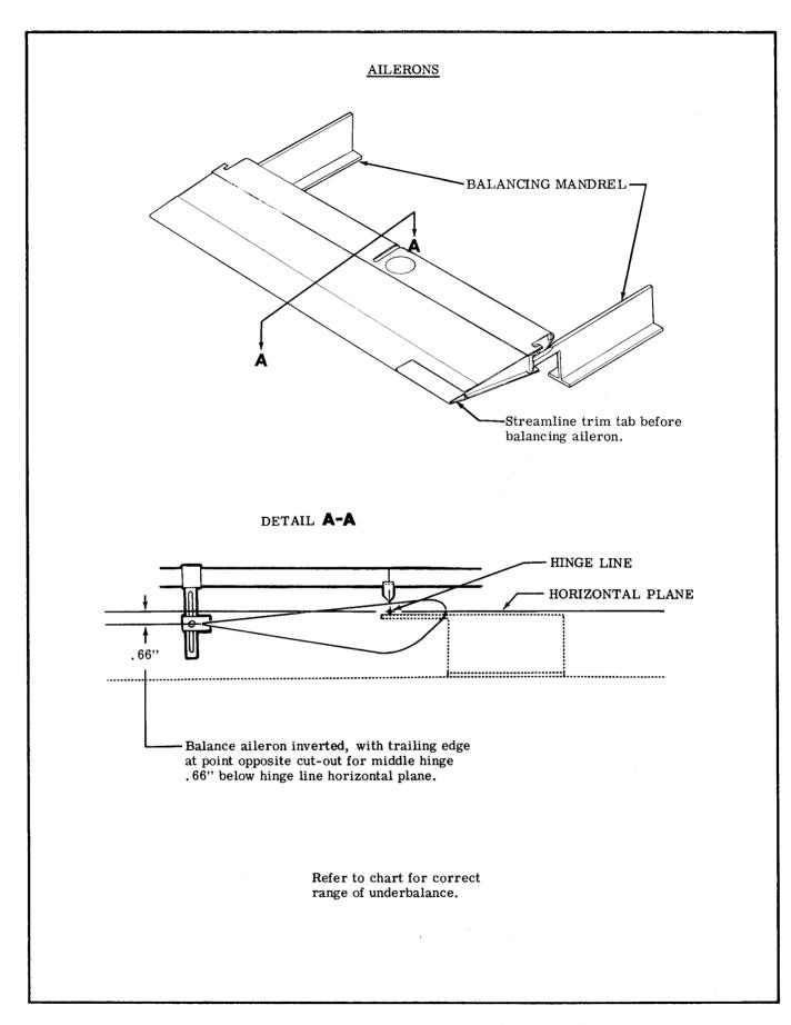
Figure 18-3. Control Surface Balancing (Sheet 3 of 4)
