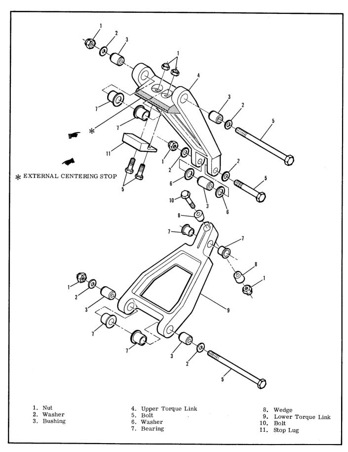
Figure 5-11. Torque Links
