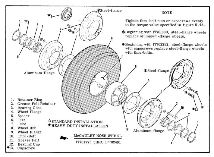
Figure 5-8. Nose Wheel (Sheet 2 of 3)
