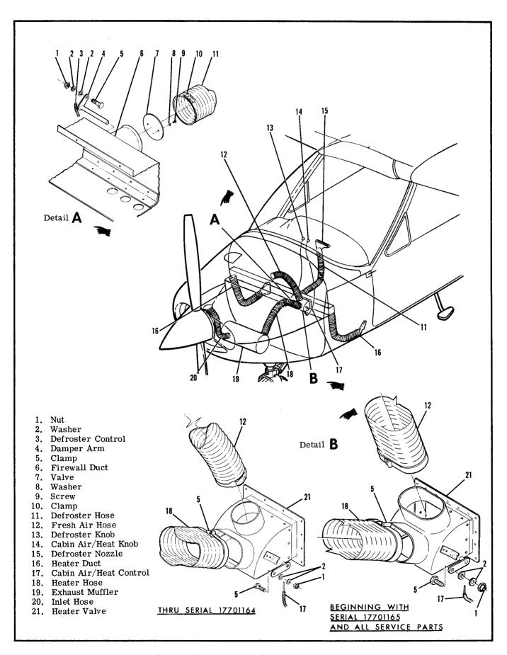
Figure 14-1. Heating and Defrosting Systems
