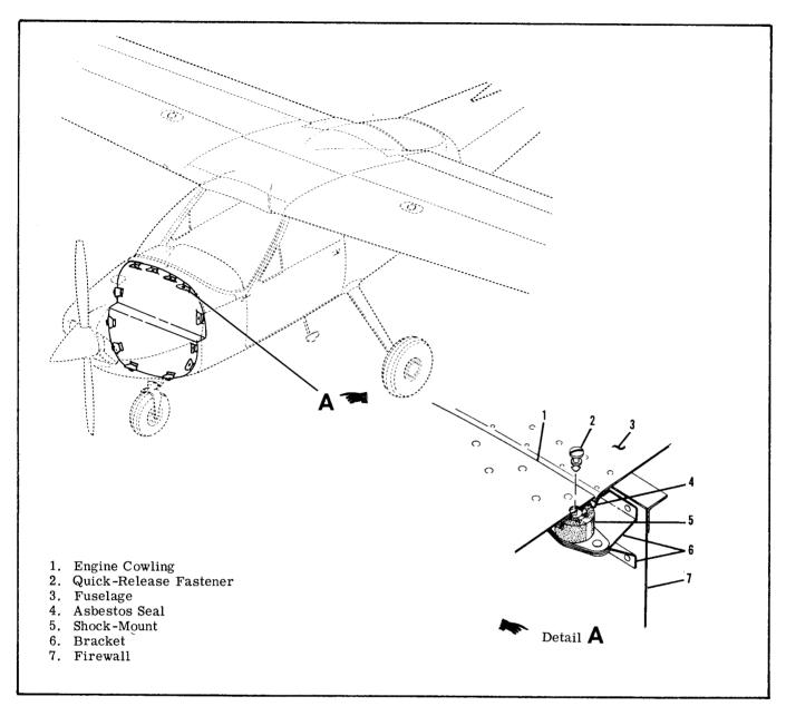
Figure 11-1. Engine Cowling Shock-Mounts
