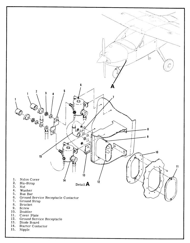
Figure 16-3. Ground Service Receptacle Installation
