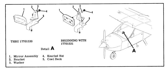
Figure 3-9. Rear View Mirror Installation
