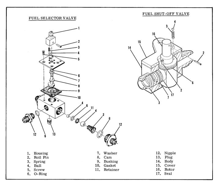
Figure 12-6. Fuel Selector Valve and Shut-Off Valve
