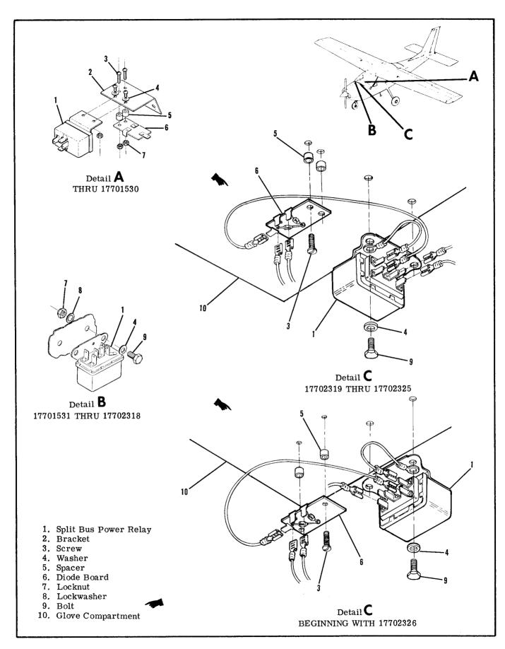
Figure 16-1. Split Bus Power Relay Installation
