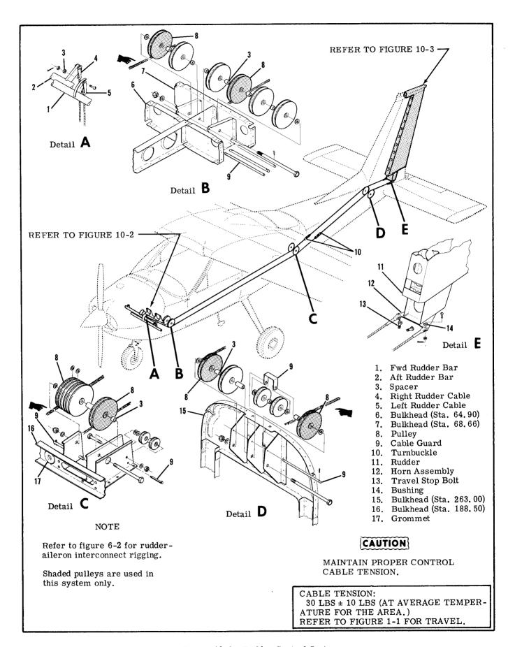
Figure 10-1. Rudder Control System
