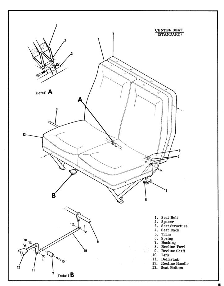
Figure 3-6. Seat Installation (Sheet 5 of 7)
