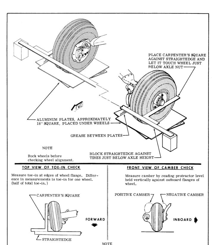
Setting toe-in and camber within these tolerances while the cabin and fuel tanks are empty will give approximately zero toe-in and zero camber at gross weight. Therefore, if normal operation is at less than gross weight and abnormal tire wear occurs, realign the wheels to attain the ideal setting for the load conditions. Refer to sheet 2 of this figure for shims availability and their usage. Always use the least number of shims possible to obtain the desired result.
