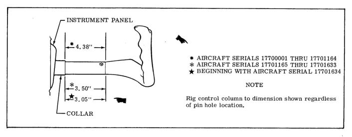
Figure 8-3. Control Column Neutral Position
