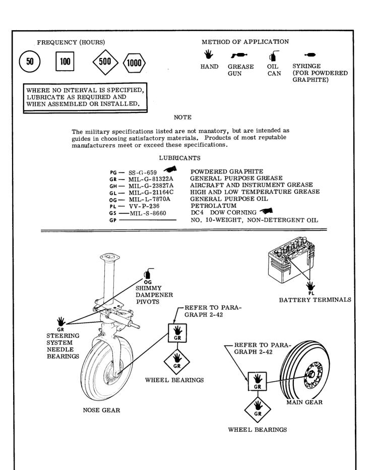
Figure 2-4. Lubrication (Sheet 1 of 3)
