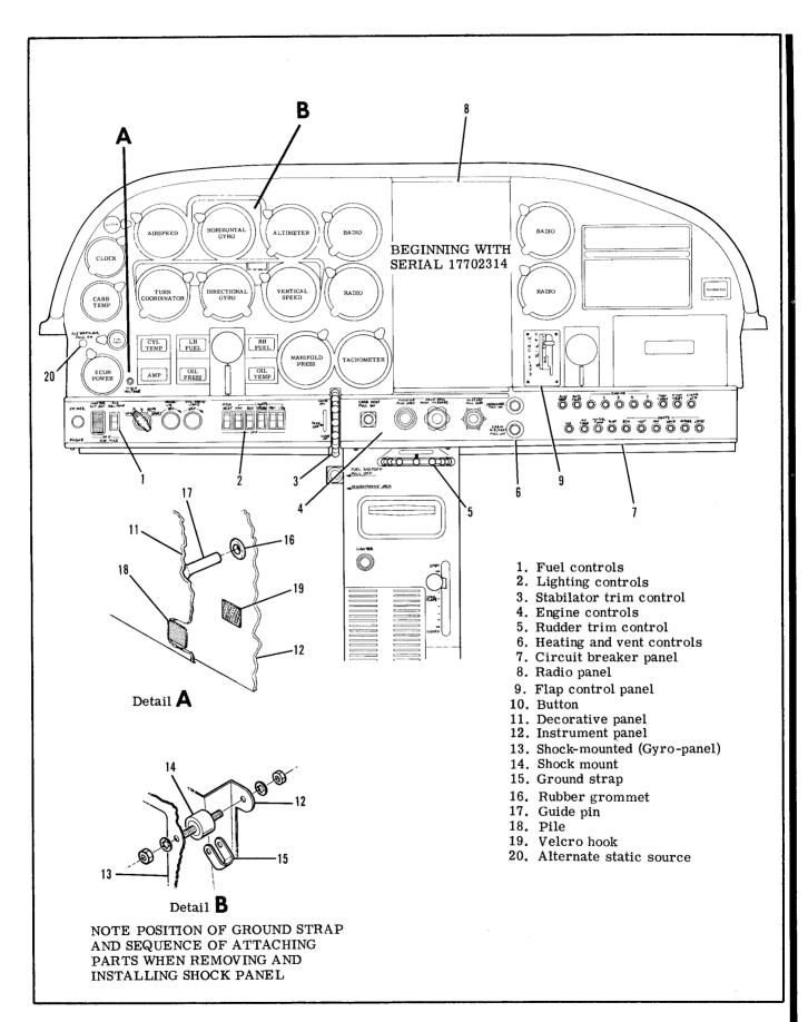
Figure 15-1. Instrument Panel (Typical) (Sheet 2 of 2)
