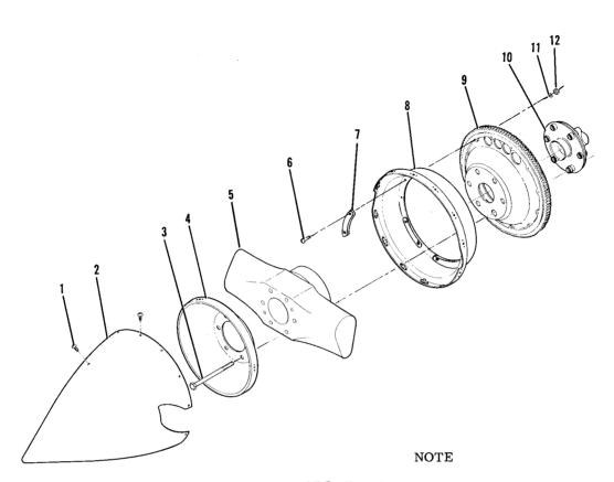
TORQUE PROPELLER MOUNTING BOLTS TO 45 LB-FT.
