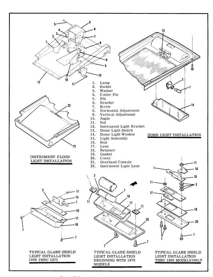
Figure 16-9. Dome and Instrument Lights Installation
