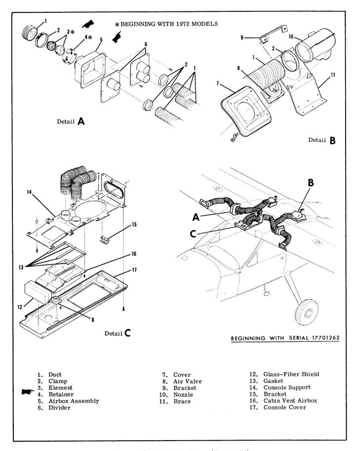
Figure 14-2. Ventilating System (Sheet 3 of 3)
