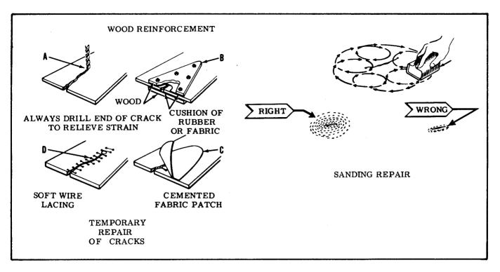
Figure 3-1. Repair of Windshield and Windows
