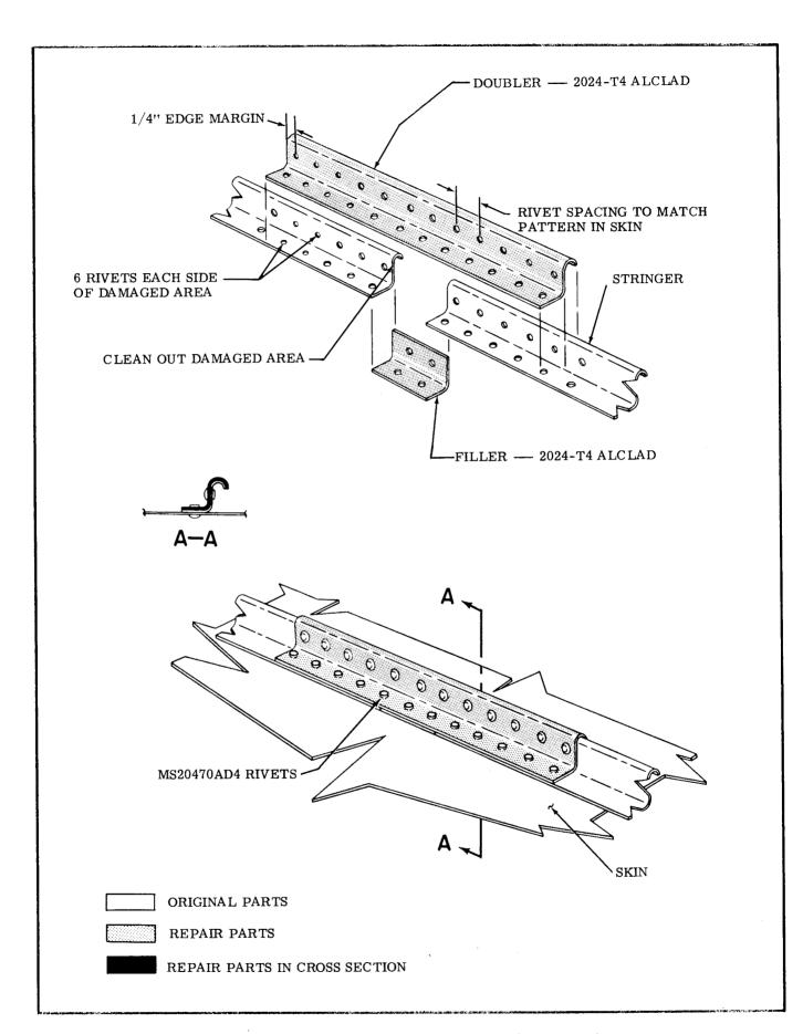
Figure 18-5. Stringer and Channel Repair (Sheet 1 of 4)
