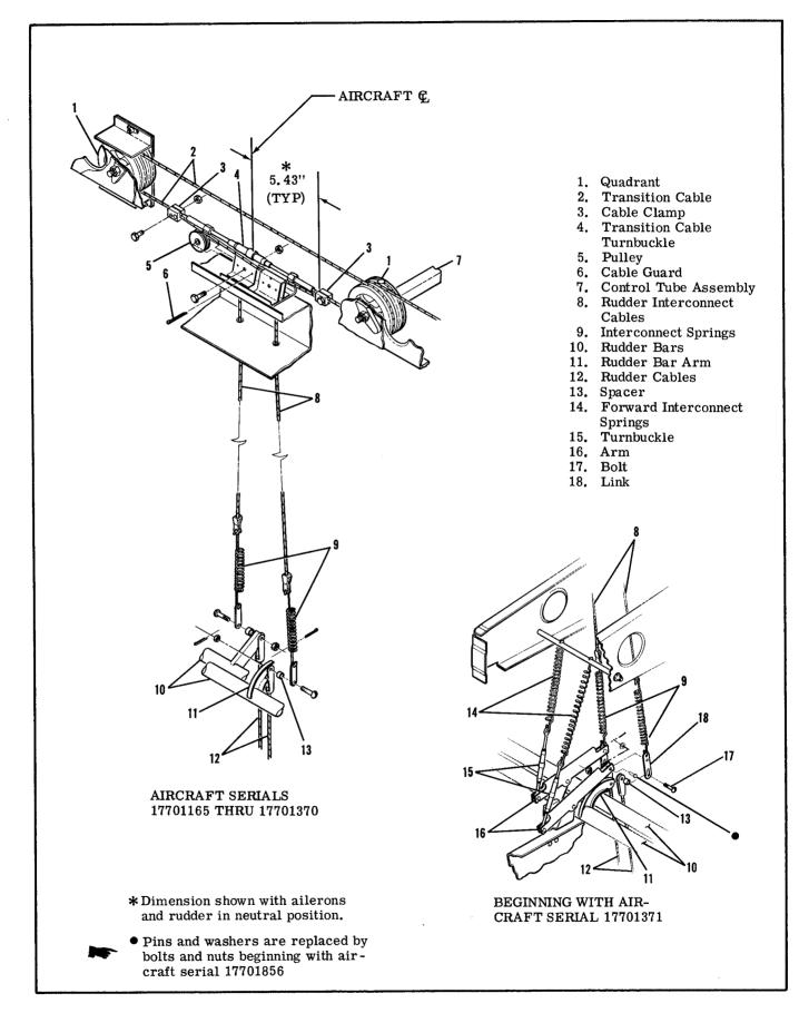
Figure 6-3. Aileron-Rudder Interconnect System
