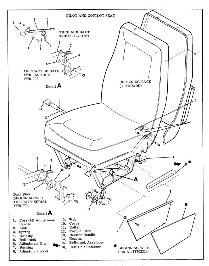
Figure 3-6. Seat Installation (Sheet 1 of 7)
