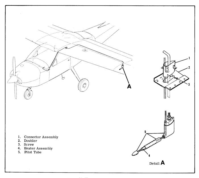
Figure 16-12. Heated Pitot Installation
