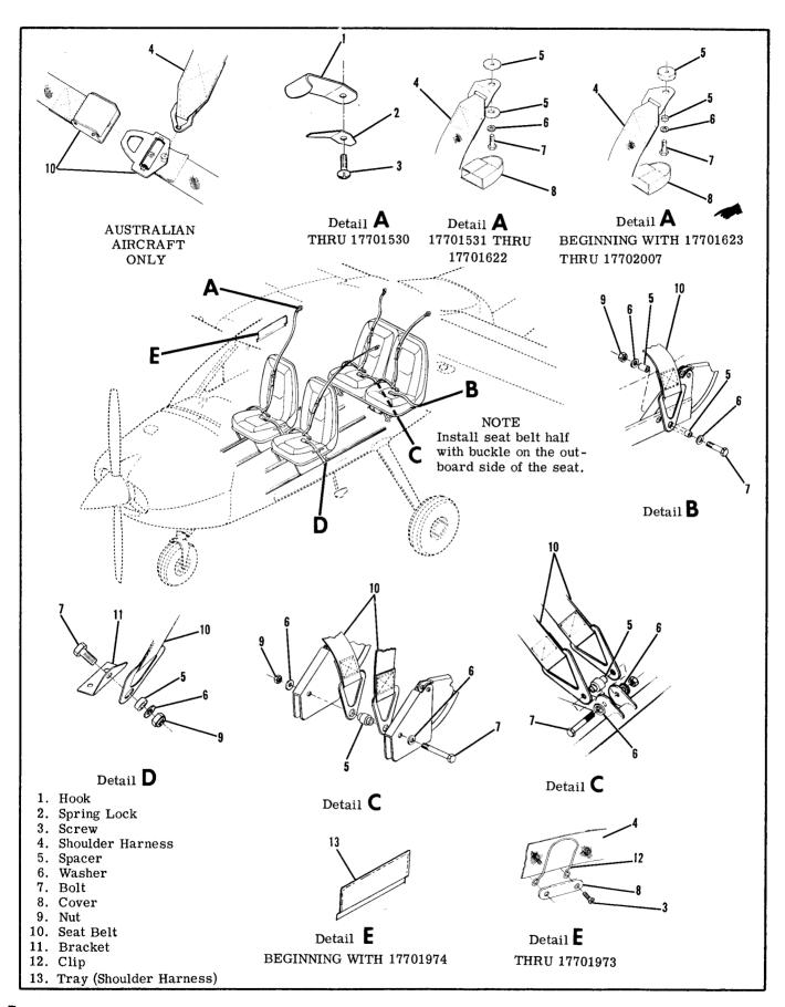
Figure 3-6A. Seat Belt and Shoulder Harness Installation(Sheet 1 of 2)
