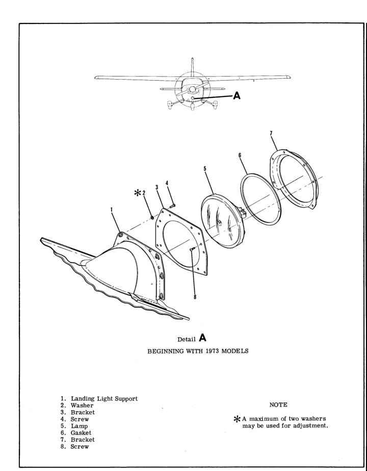
Figure 16-6. Landing and Taxi Light Installation (Sheet 3 of 3)
