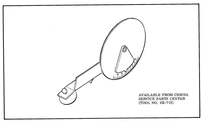
Figure 6-5. Inclinometer for Measuring Control Surface Travels
