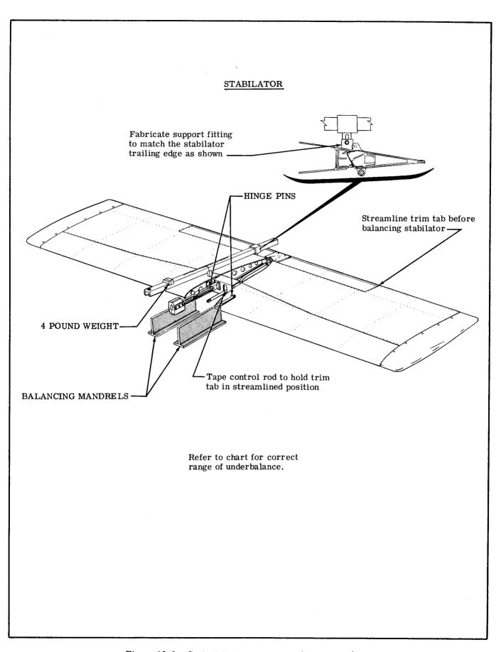
Figure 18-3. Control Surface Balancing (Sheet 4 of 4)
