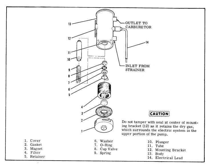
Figure 12-8. Electric Fuel Pump
