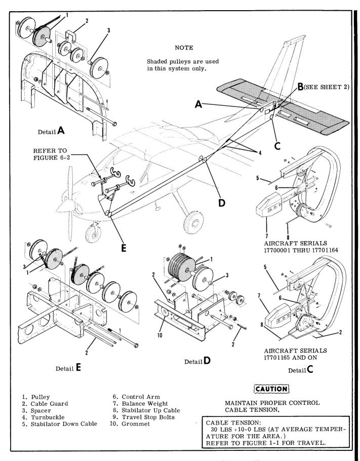
Figure 8-1. Stabilator Control System (Sheet 1 of 2)
