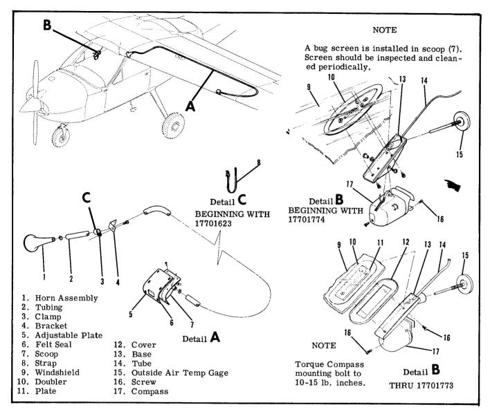
Figure 15-6. Stall Warning and Outside Air Temperature Gage Installation.
