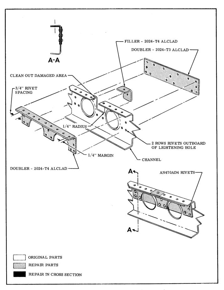
Figure 18-5. Stringer and Channel Repair (Sheet 4 of 4)
