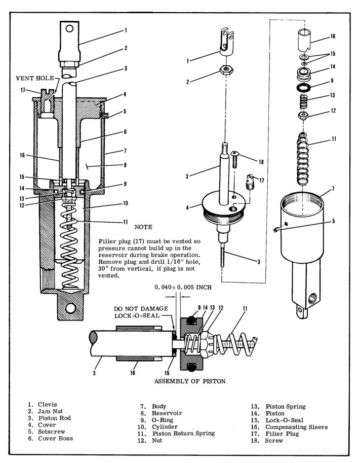
Figure 5-13. Brake Master Cylinder
