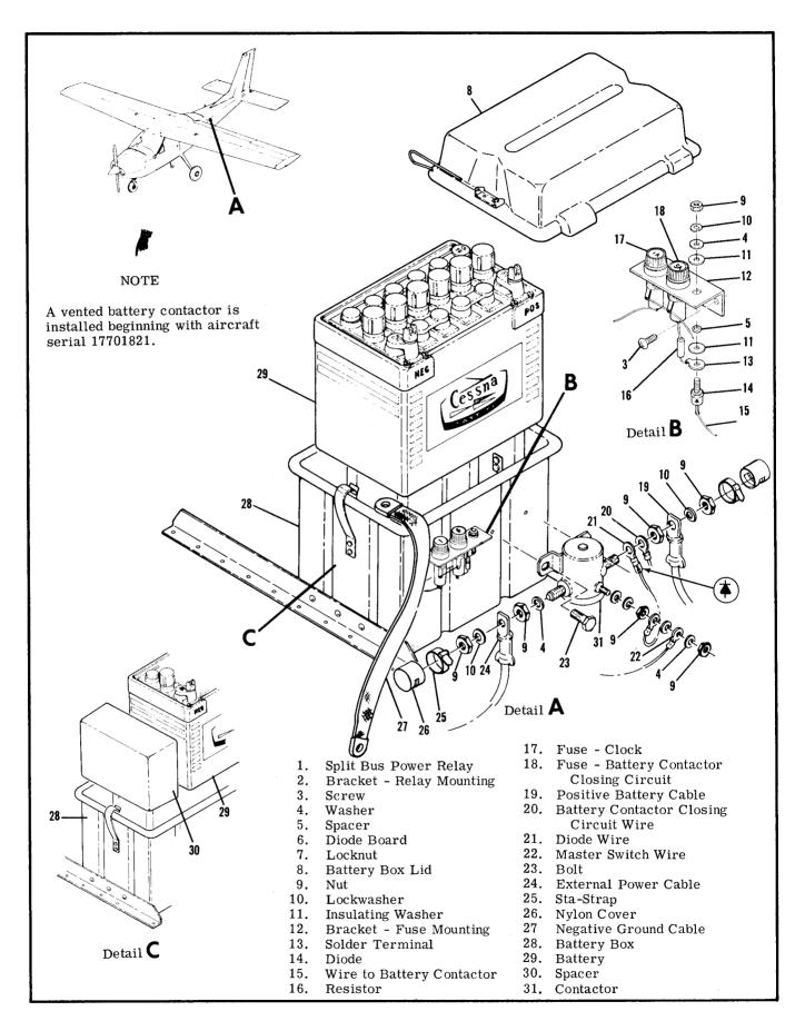
Figure 16-2. Battery and Electrical Equipment Installation
