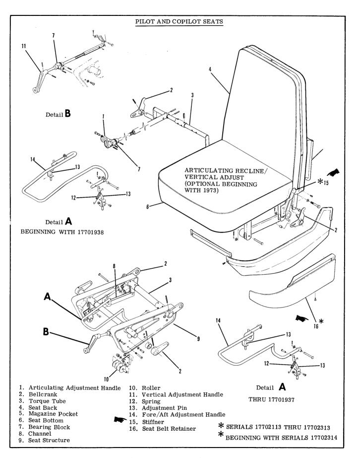
Figure 3-6. Seat Installation (Sheet 4 of 7)
