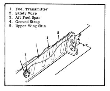
Figure 15-6A. Ground Strap Installation
