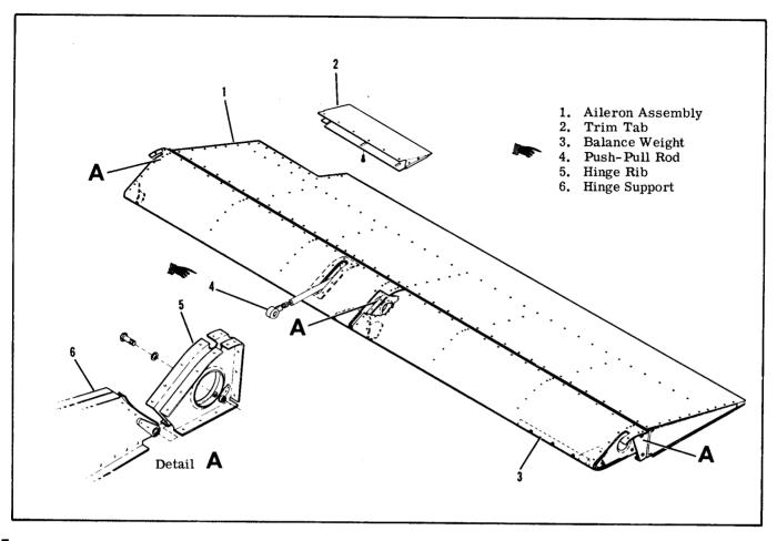
Figure 6-4. Aileron Installation
