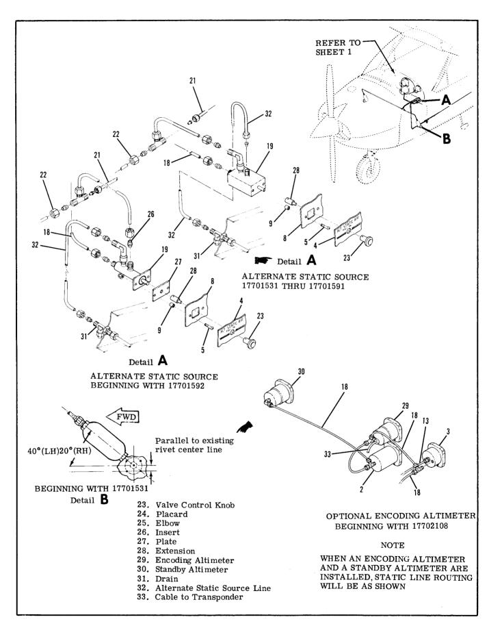
Figure 15-2. Pitot Static Systems (Sheet 2 of 2)
