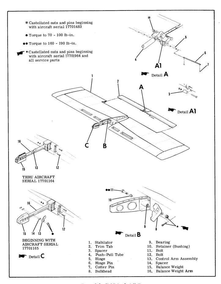
Figure 8-2. Stabilator Installation
