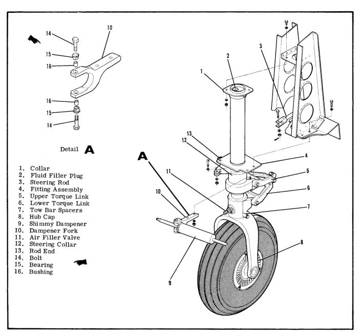
Figure 5-6. Nose Gear Installation
