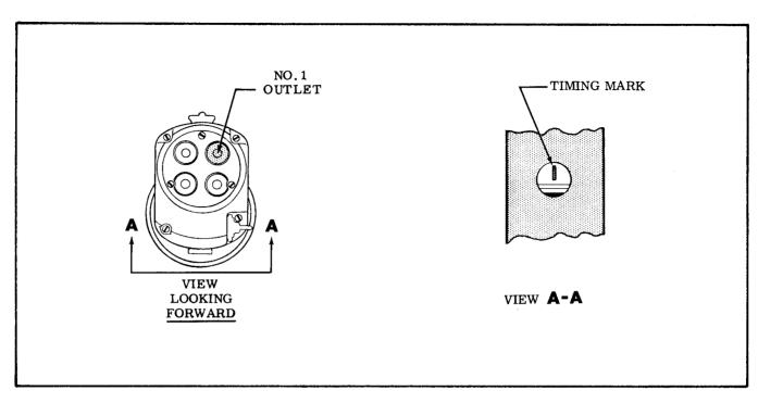
Figure 11-4. Magneto Outlet
