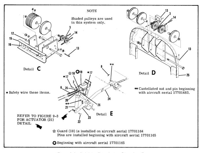
Figure 9-1. Stabilator Trim System (Sheet 2 of 2)
