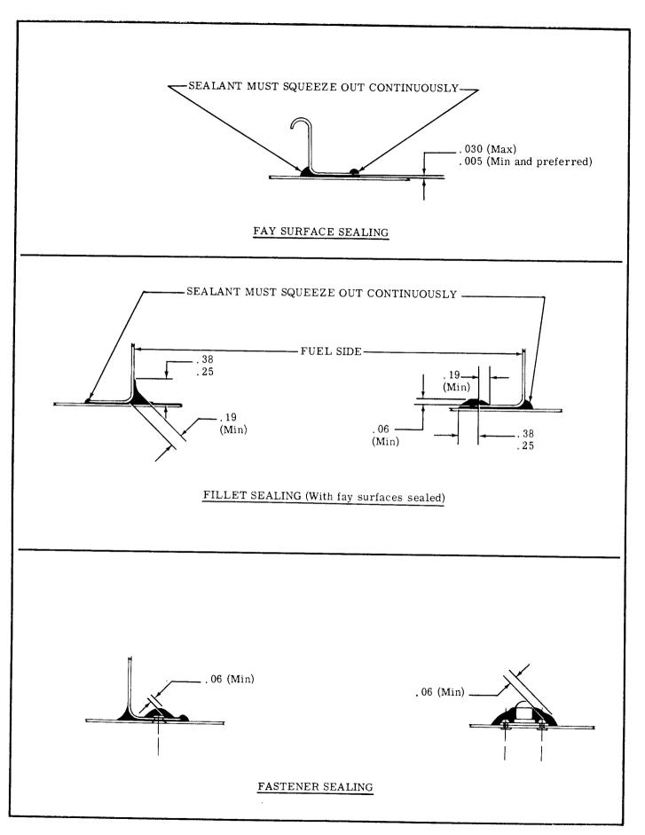
Figure 12-5. Fuel Bay Sealing (Sheet 2 of 2)
