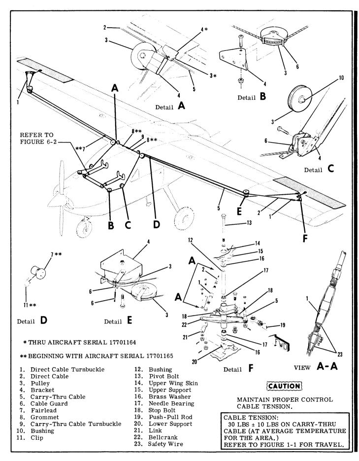
Figure 6-1. Aileron Control System
