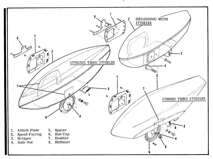
Figure 5-2. Main Wheel Speed Fairing
