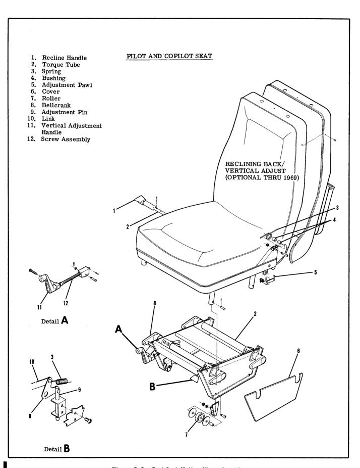
Figure 3-6. Seat Installation (Sheet 2 of 7)
