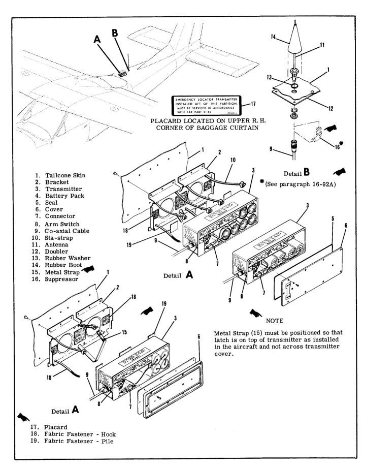
Figure 16-14. Emergency Locator Transmitter Installation
