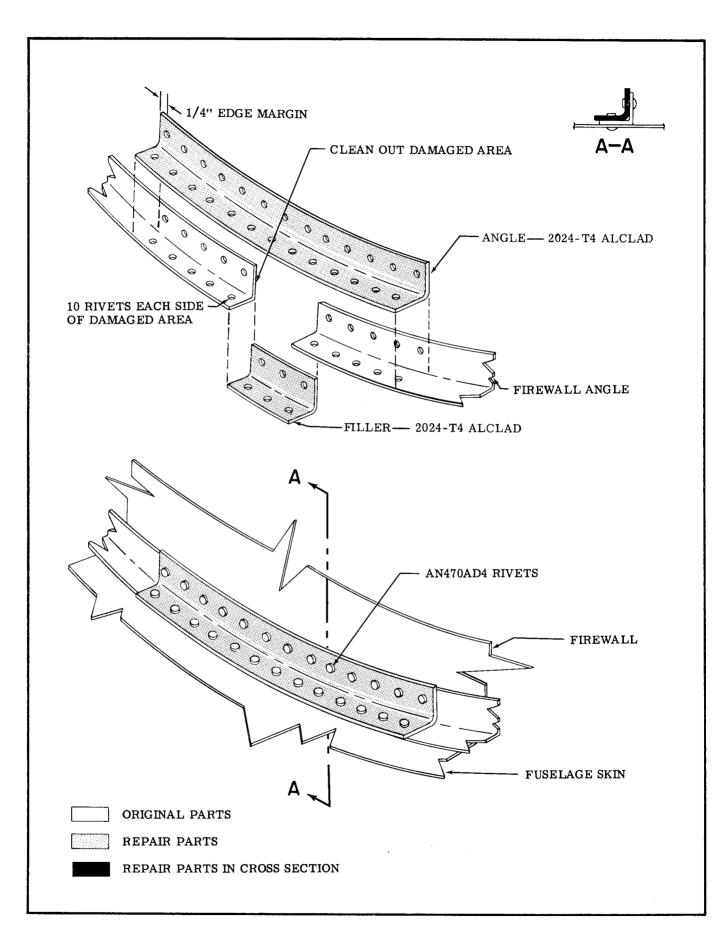
Figure 18-11. Firewall Angle Repair
