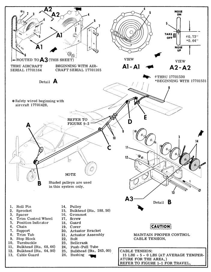
Figure 9-1. Stabilator Trim System (Sheet 1 of 2)
