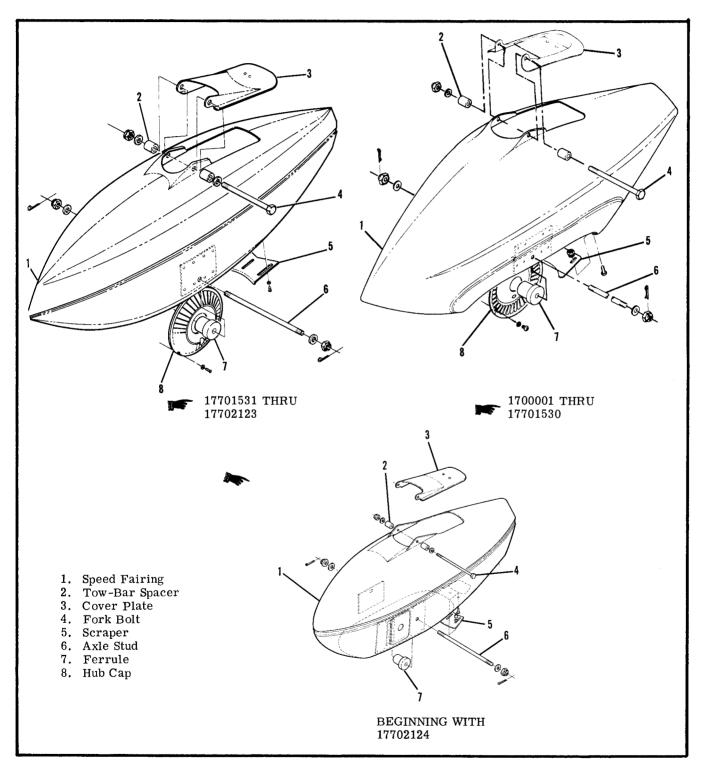
Figure 5-7. Nose Wheel Speed Fairing
