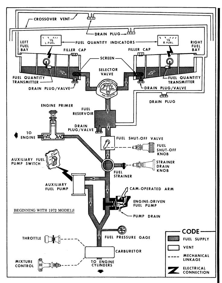
Figure 12-1A. Fuel System Schematic
