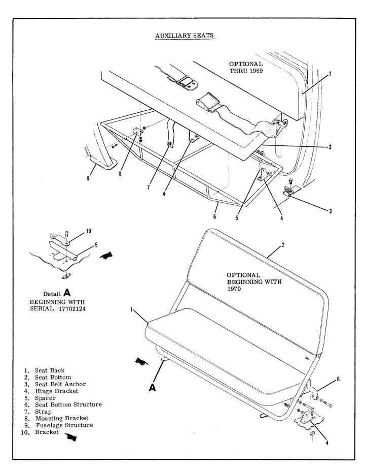
Figure 3-6. Seat Installation (Sheet 7 of 7)
