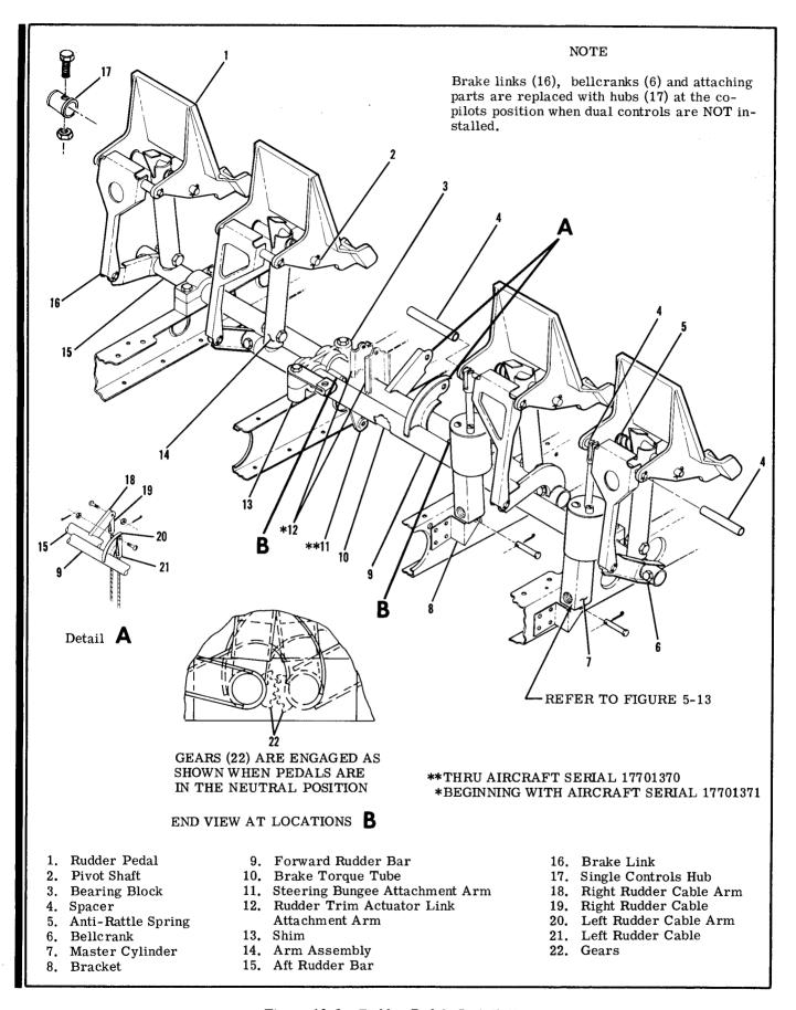
Figure 10-2. Rudder Pedals Installation
