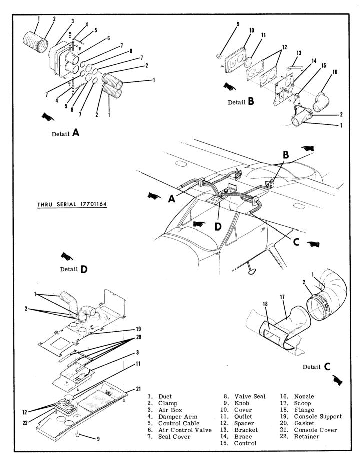
Figure 14-2. Ventilating System (Sheet 1 of 3)
