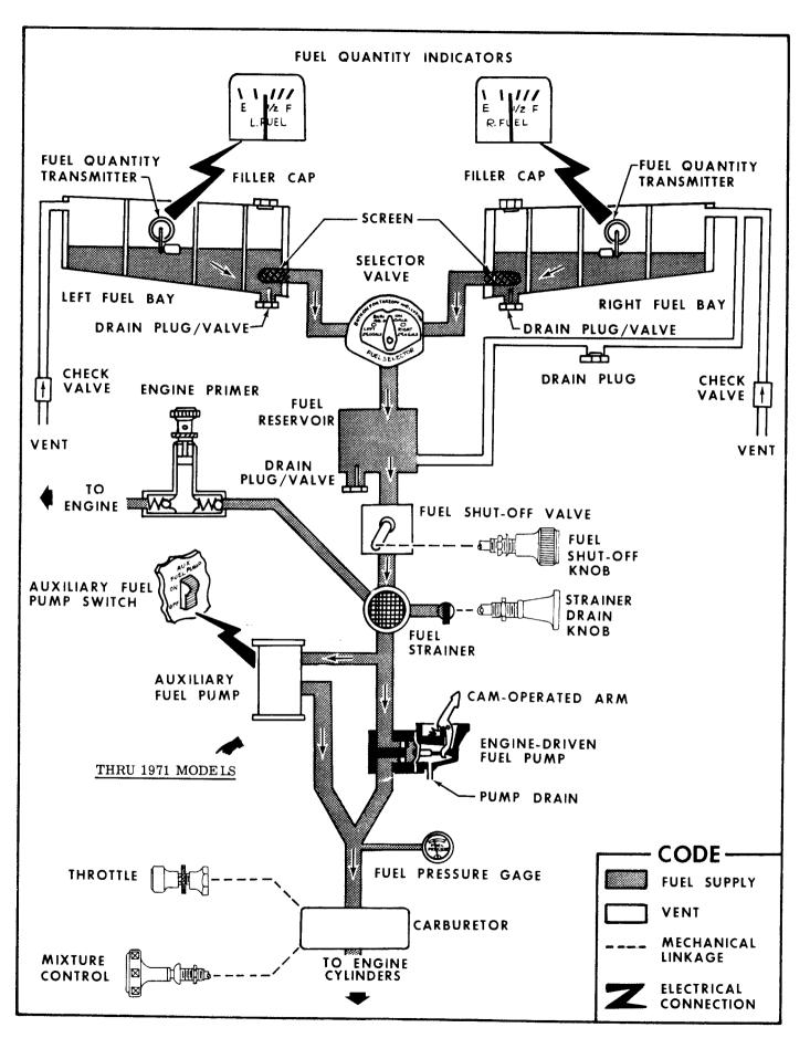
Figure 12-1. Fuel System Schematic
