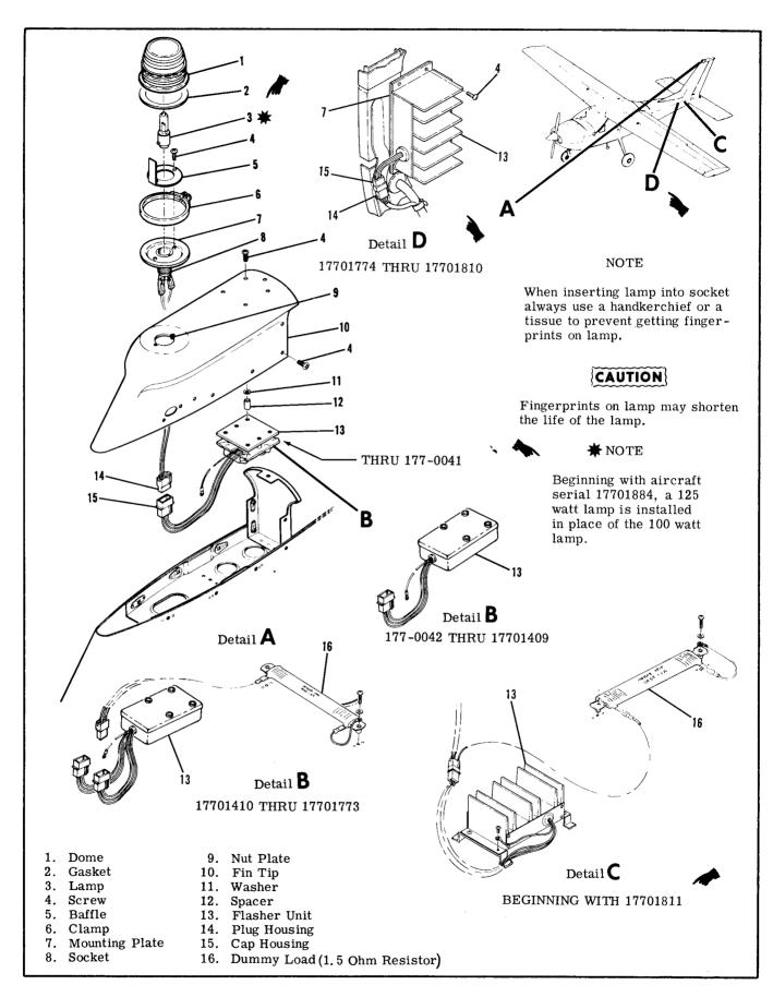
Figure 16-8. Flashing Beacon Light Installation
