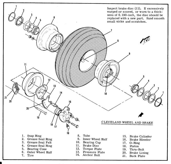
Figure 5-4. Cleveland Wheel and Brake Assembly
