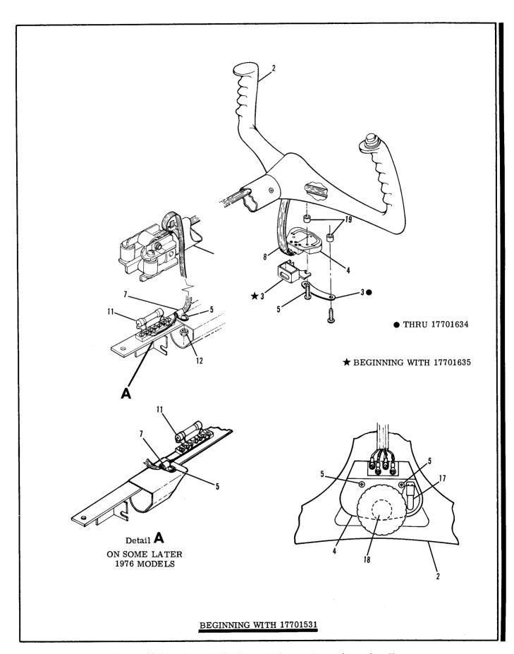
Figure 16-11. Control Wheel Map Light Installation (Sheet 2 of 2)
