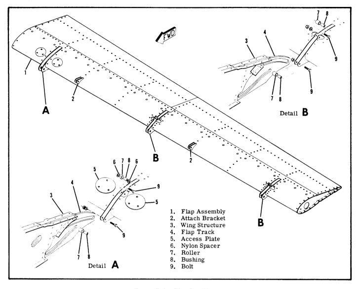
Figure 7-3. Flap Installation
