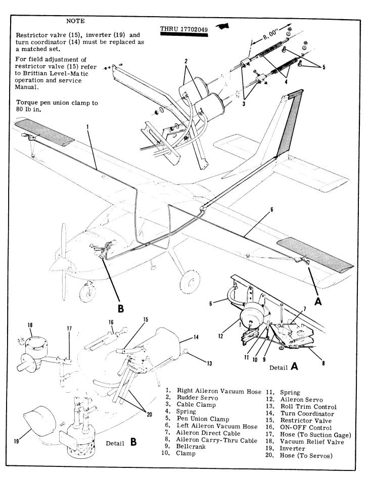
Figure 15-8. Wing Leveler Control System
