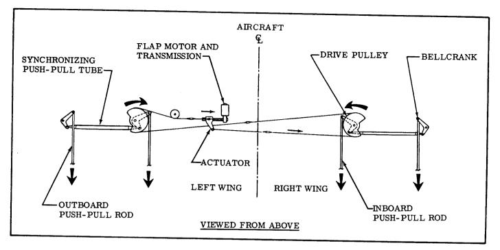
Figure 7-4. Flap System Schematic
