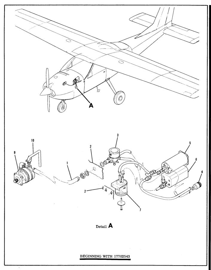
Figure 15-5. Vacuum System (Typical) (Sheet 2 of 2)
