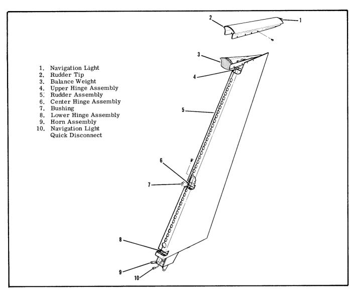
Figure 10-3. Rudder Assembly
