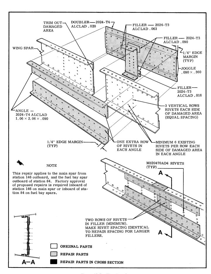
Figure 18-7. Wing Spar Repair
