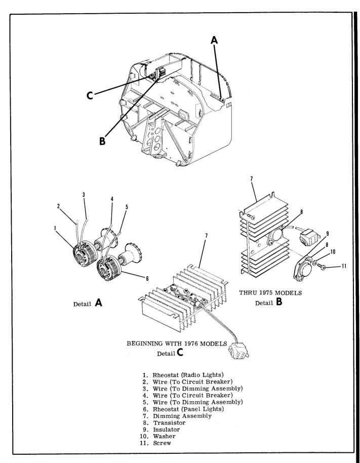
Figure 16-10A. Transistorized Light Dimming Installation
