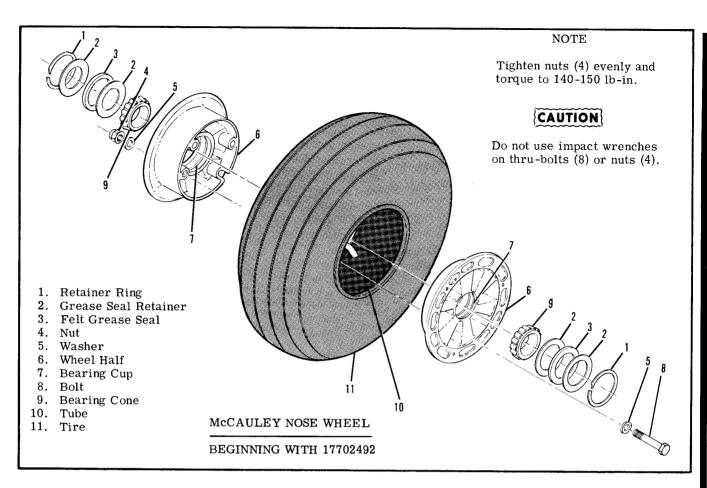
Figure 5-8. Nose Wheel (Sheet 3 of 3)
