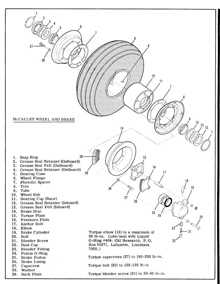
Figure 5-4A. McCauley Wheel and Brake Assembly
