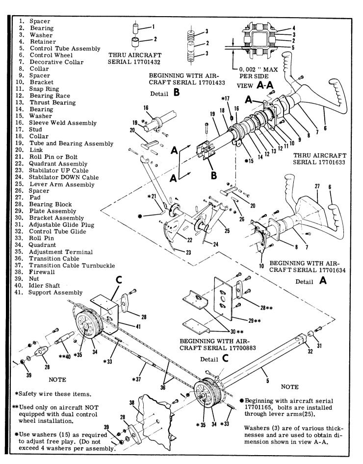
Figure 6-2. Control Column Installation
