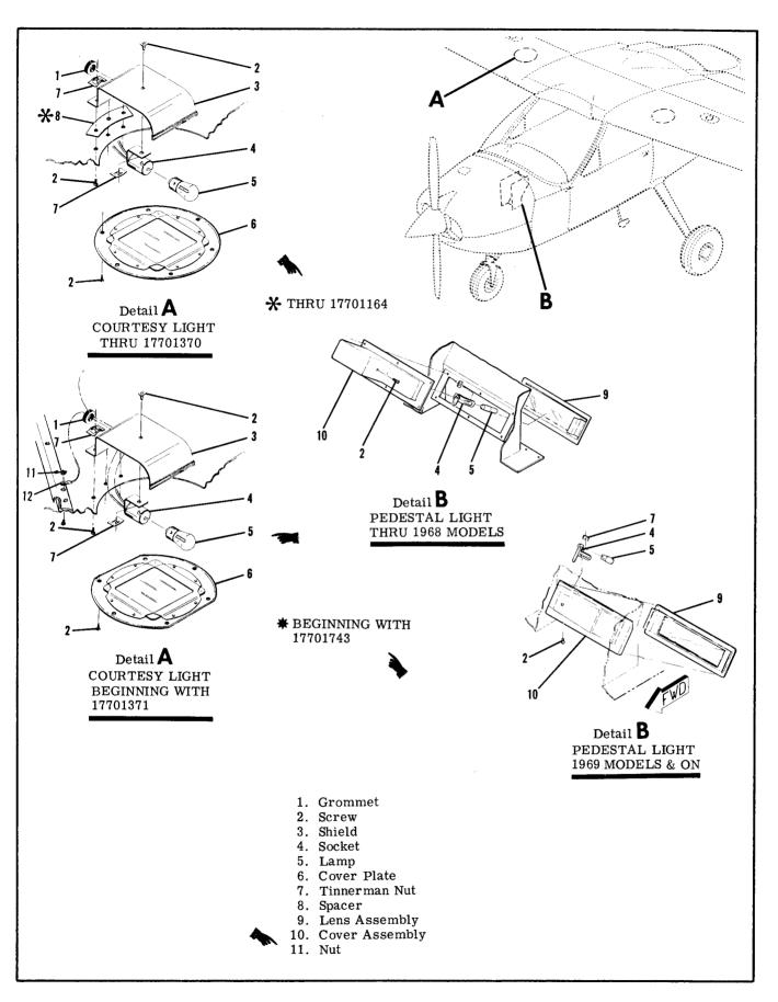
Figure 16-10. Courtesy Lights Installation
