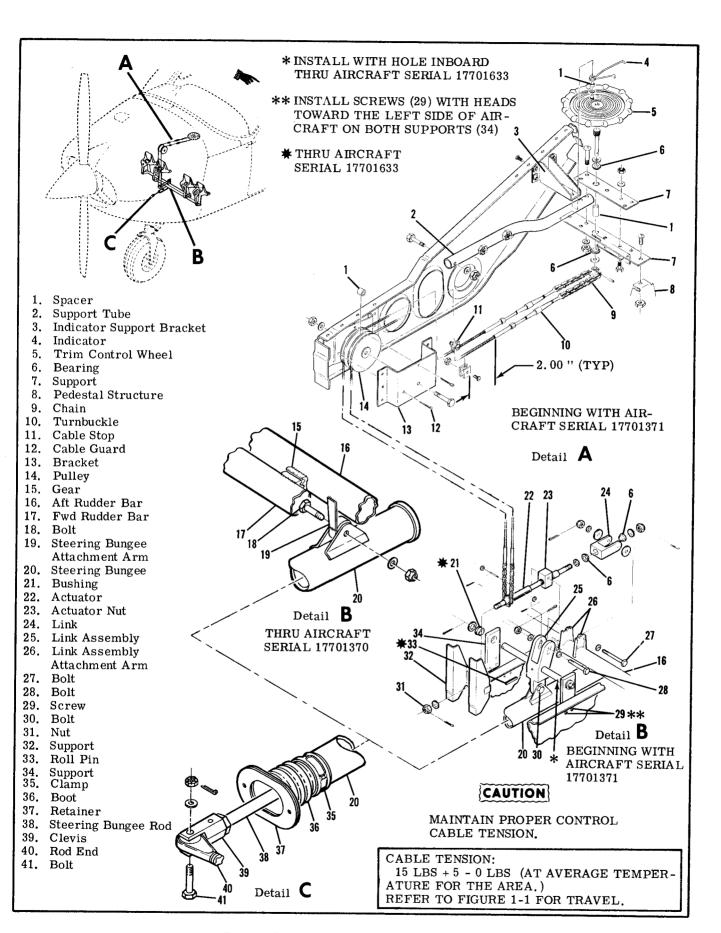
Figure 10-5. Rudder Trim Control System
