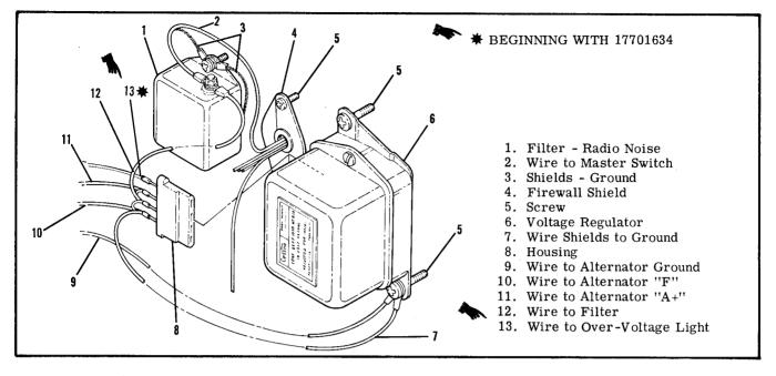
Figure 16-5. Voltage Regulator Installation
