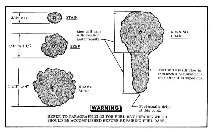
Figure 12-4. Classification of Fuel Leaks
