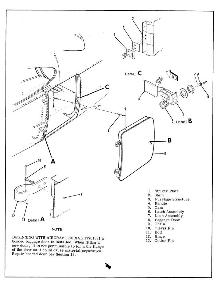
Figure 3-5. Baggage Door Installation
