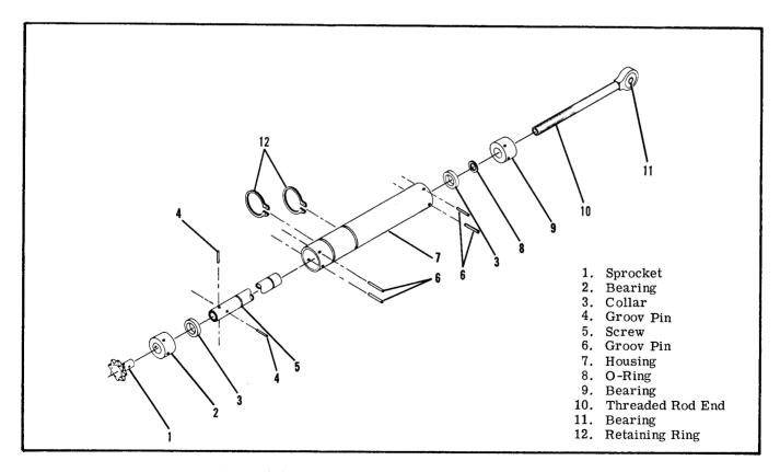
Figure 9-3. Stabilator Trim Tab Actuator Assembly
