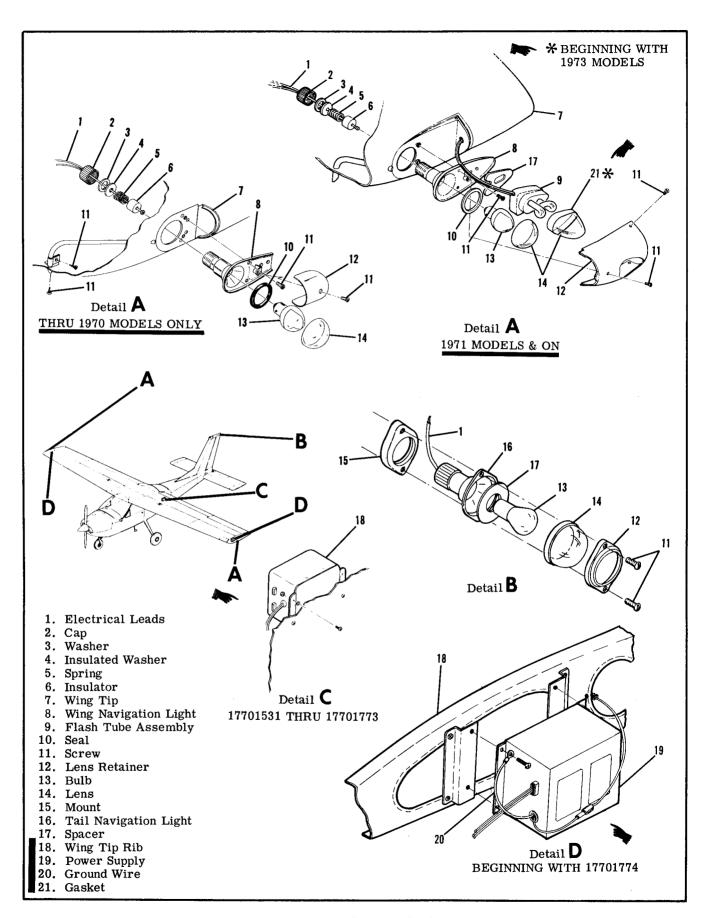
Figure 16-7. Navigation and Anti-Collision Strobe Lights Installation
