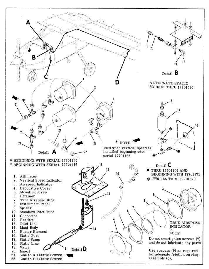
Figure 15-2. Pitot Static Systems (Sheet 1 of 2)
