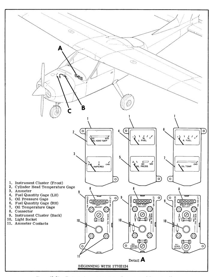
Figure 15-5A. Engine Instrument Installation (Leigh System) (Sheet 1 of 2)
