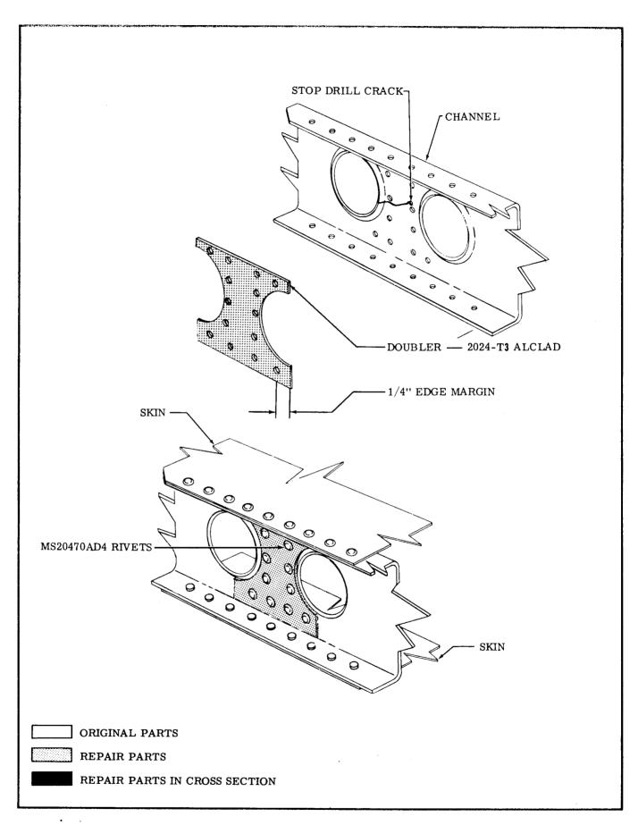
Figure 18-5. Stringer and Channel Repair (Sheet 3 of 4)
