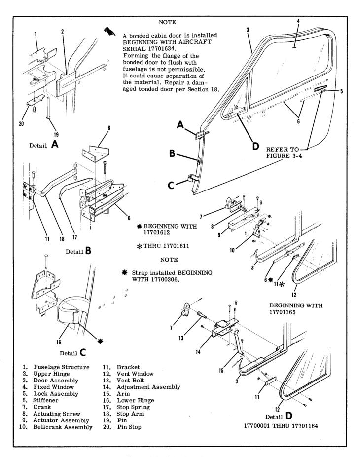
Figure 3-3. Cabin Door Installation
