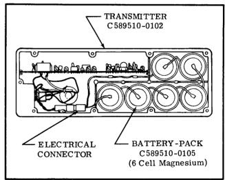
Figure 16-15. Magnesium 6 Cell Battery-Pack Installation
