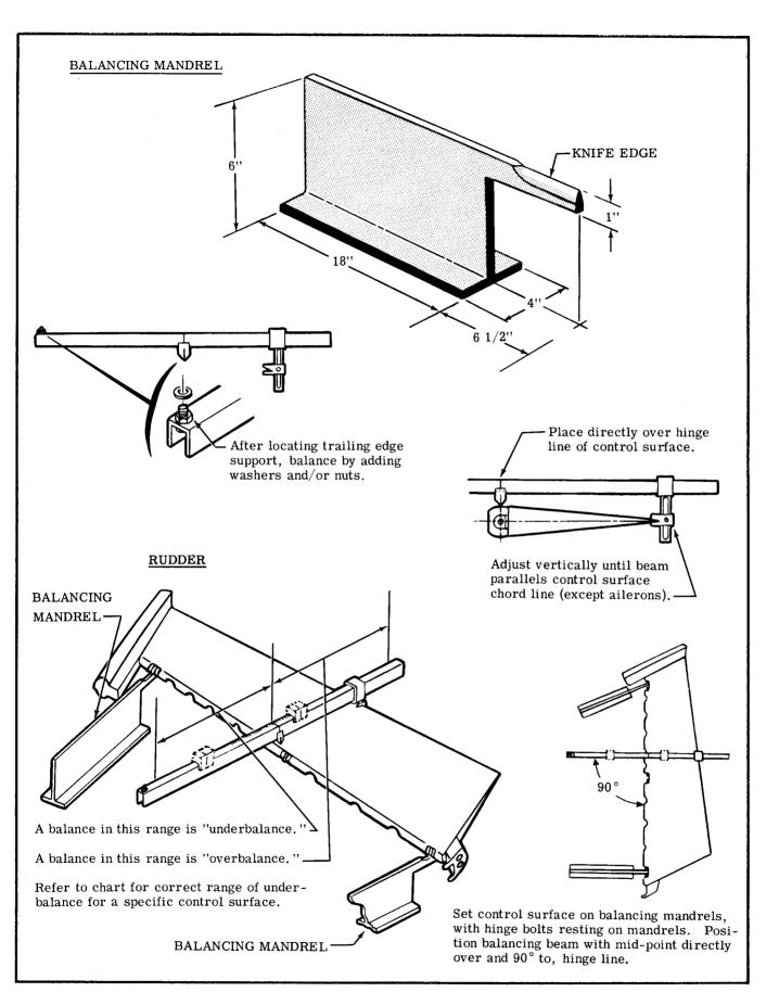
Figure 18-3. Control Surface Balancing (Sheet 2 of 4)
