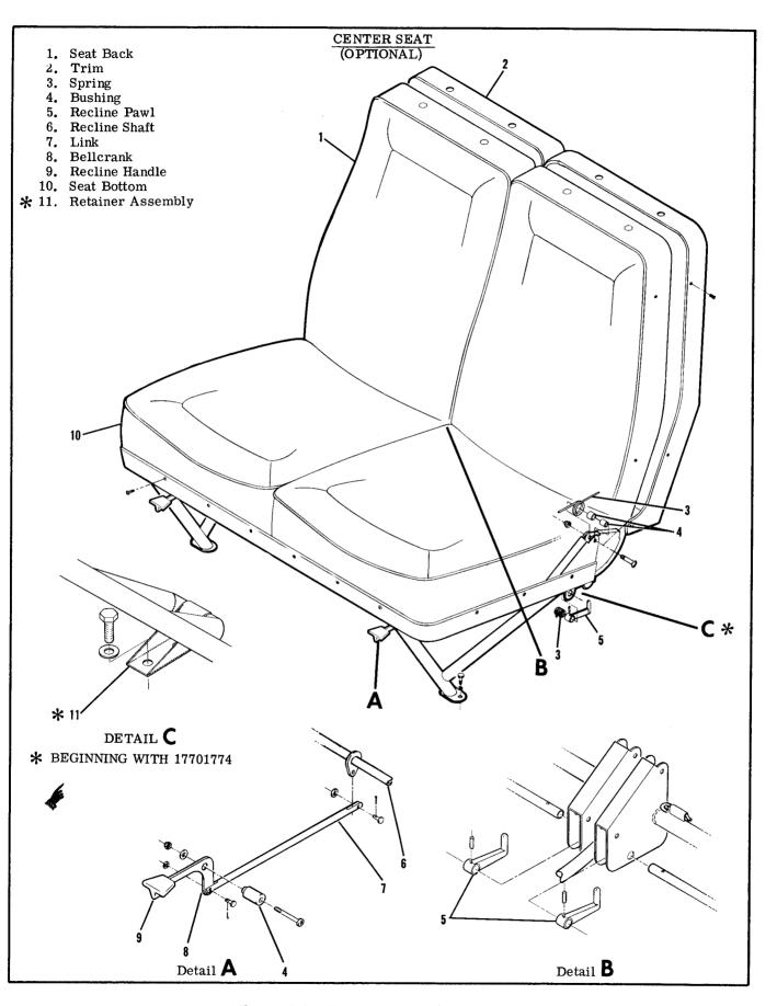
Figure 3-6. Seat Installation (Sheet 6 of 7)
