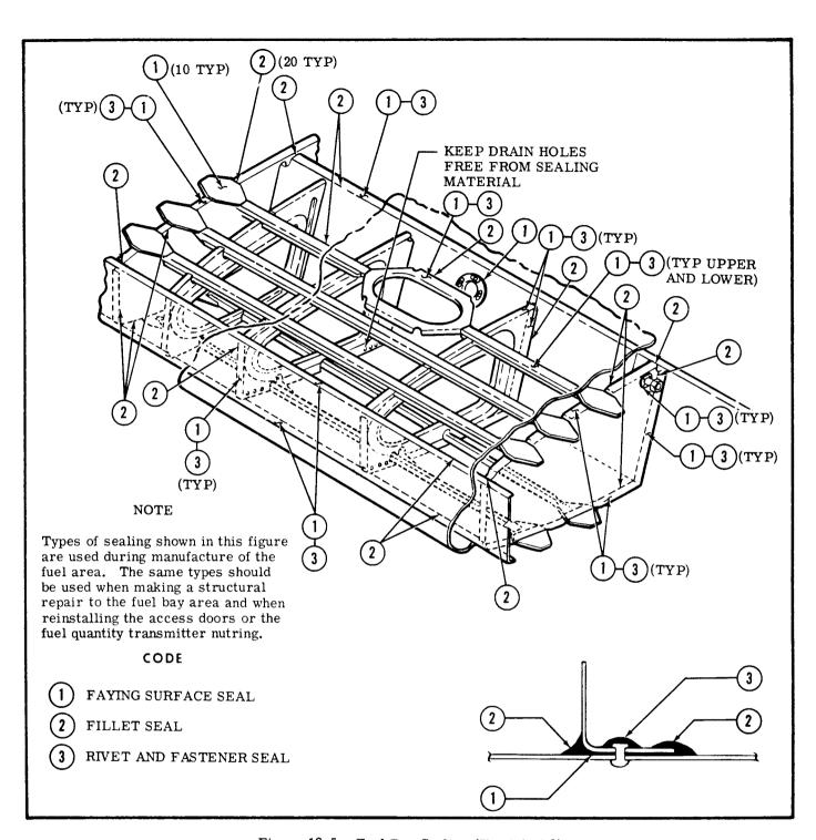
Figure 12-5. Fuel Bay Sealing (Sheet 1 of 2)
