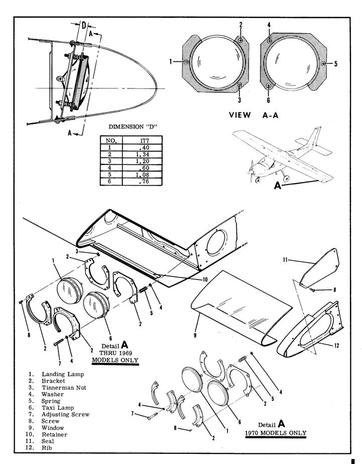
Figure 16-6. Landing and Taxi Light Installation (Sheet 1 of 3)
