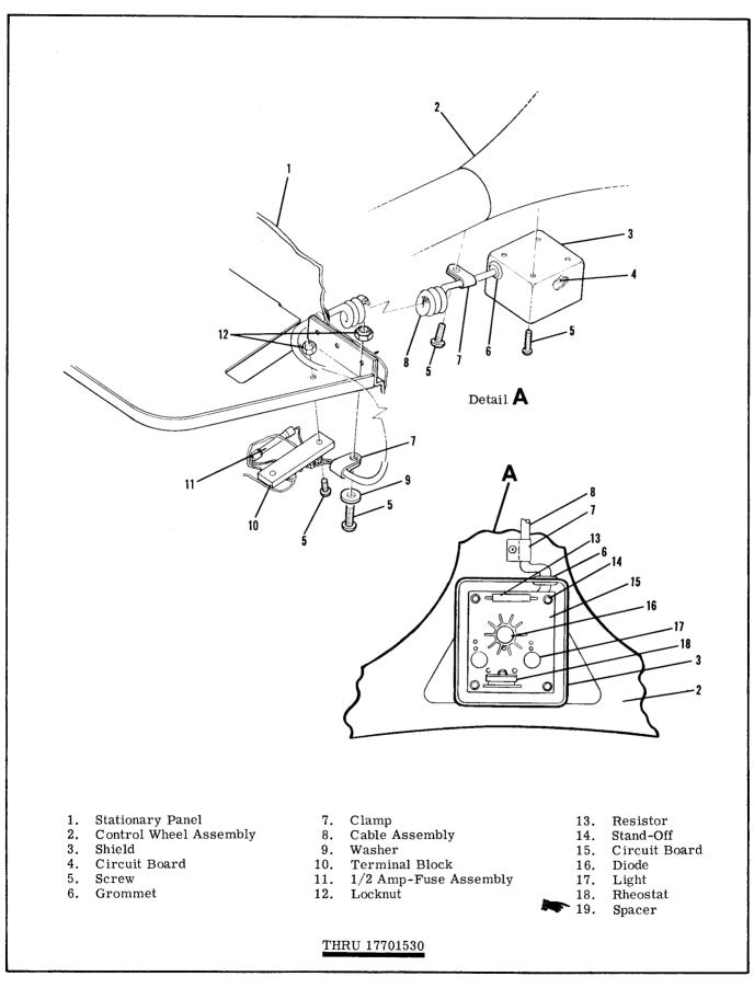
Figure 16-11. Control Wheel Map Light Installation (Sheet 1 of 2)
