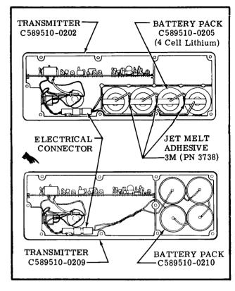
Figure 16-16. Lithium 4 Cell Battery Pack Installations
