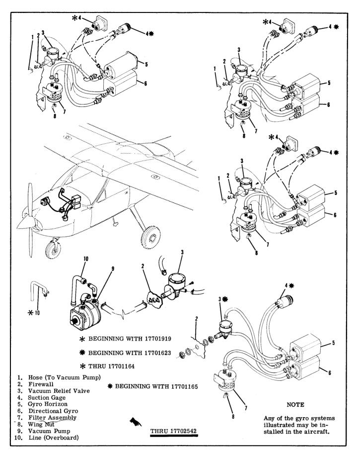
Figure 15-5. Vacuum System (Typical) (Sheet 1 of 2)
