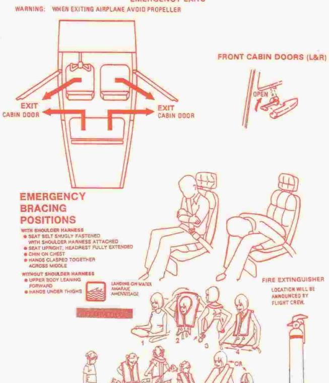
To Operate: Hold spright-Pull pin - Press lever handle Discharge at base of flame With side to side motion.
